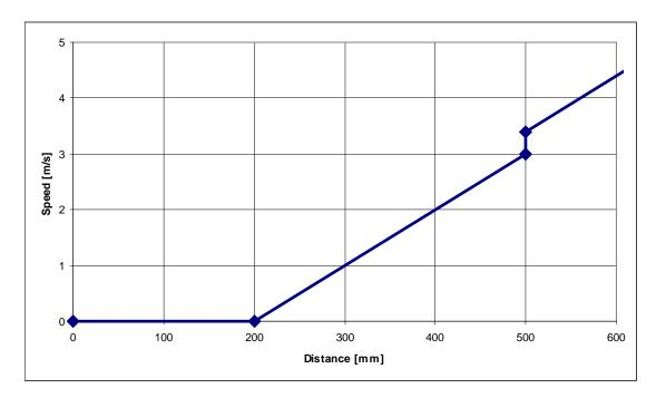
Figure 7: Graph "current distance - maximum permitted speed" for a response time of 100 ms
