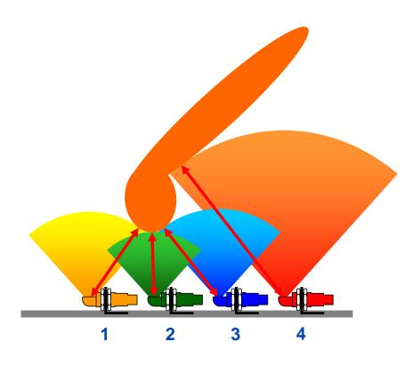
Figure 4: Penetration object throws back echoes; sensor 2 is measuring the minimum distance
