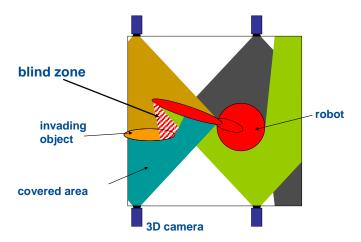
Figure 1: Workspace, monitored from without by cameras
