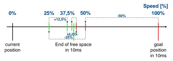
Figure 9: Trajectory based calculation of the current maximum speed
