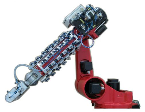
Figure 3: Reis robot with microsonic sensors
