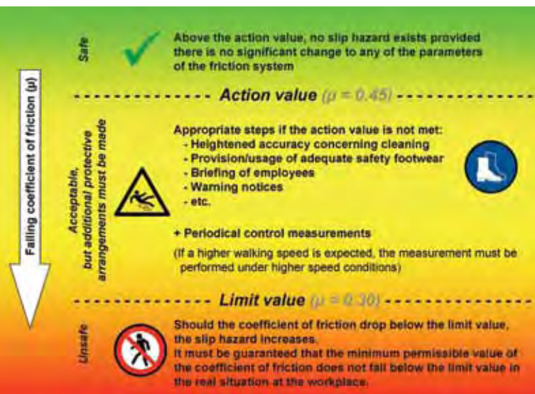
Fig. 4: Protection concept: “Action value and limit value of the coefficient of friction while walking”; Sebald, J. 2009
