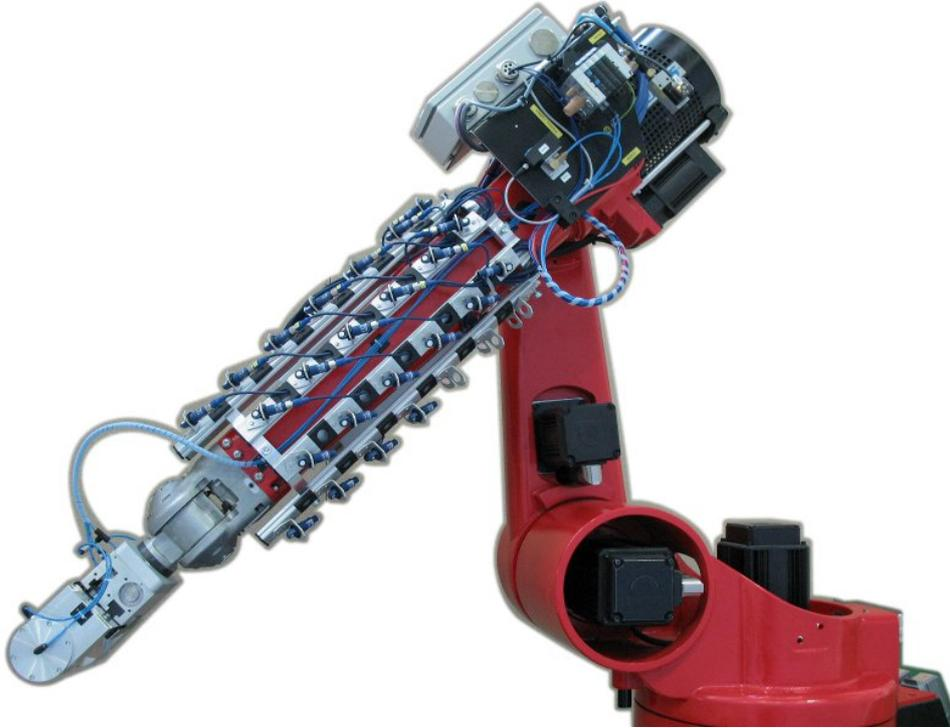
**Figure 3:** Reis robot with microsonic sensors
