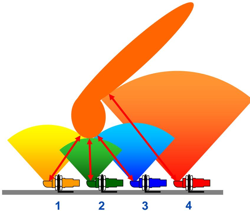
**Figure 4:** Penetration object throws back echoes; sensor 2 is measuring the minimum distance
