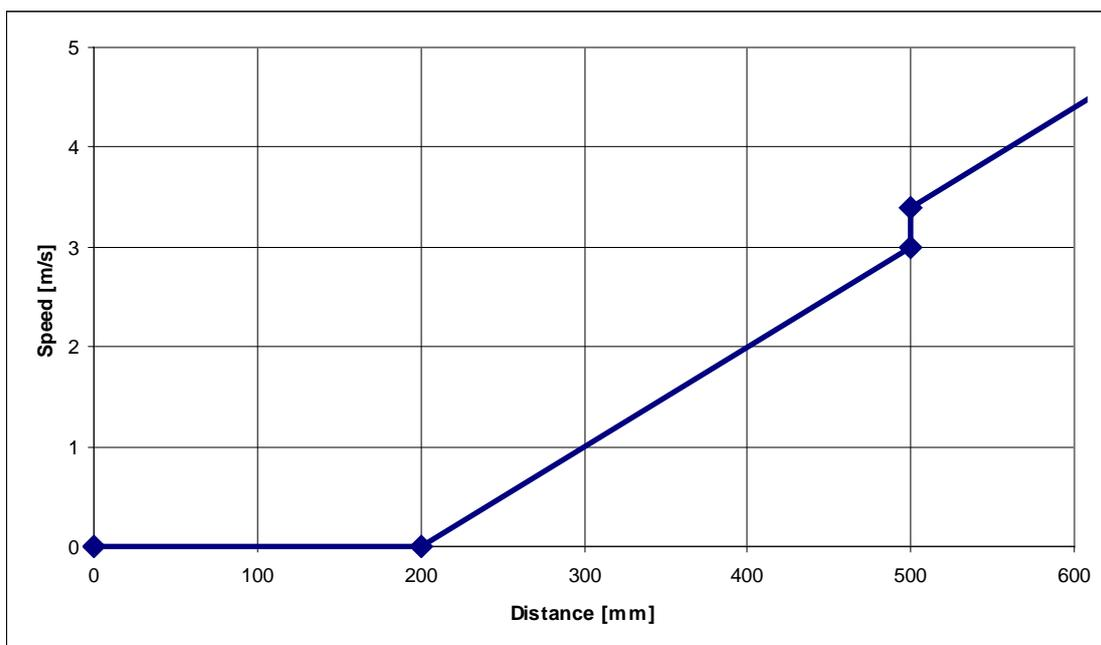
**Figure 7:** Graph "current distance - maximum permitted speed" for a response time of 100 ms
